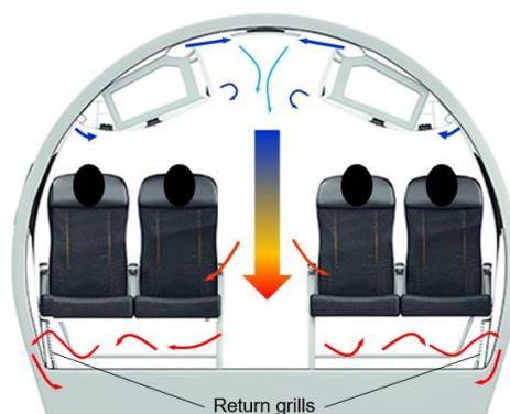
Figure 4: Airflow inside E-Jet cross-section
